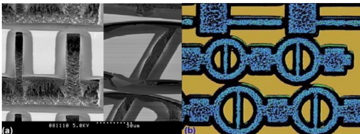
Fig. 2.11. Silicon dioxide under-etching: (a) SEM image of test structure showing the effects of RIE on the metal structure (gray areas are bent metal). (b) Confocal image of the same structure (the black borders correspond to bent metal areas)
