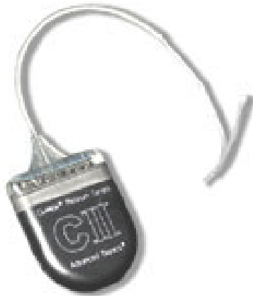
Figure 1-2. Commercial Cochlear implant. Courtesy of Advanced Bionics Corp. Figure 1-3. Expression of joy/surprise of a little girl the first time she heard a sound.
