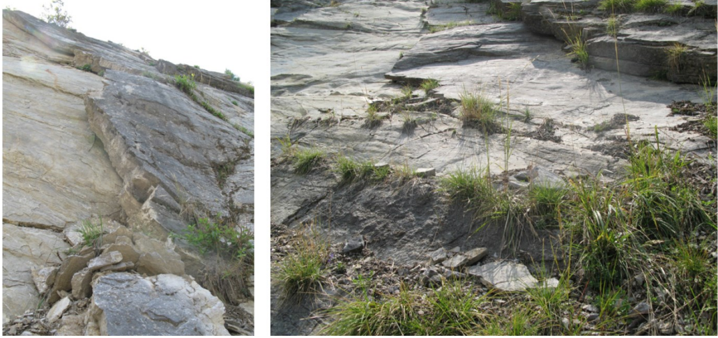
Figure 5.4: Exposed basal surface of Vajont landslide in 2007. Photographs taken in the lower part of the exposed sliding surface. (Pinyol et al., 2017a)
