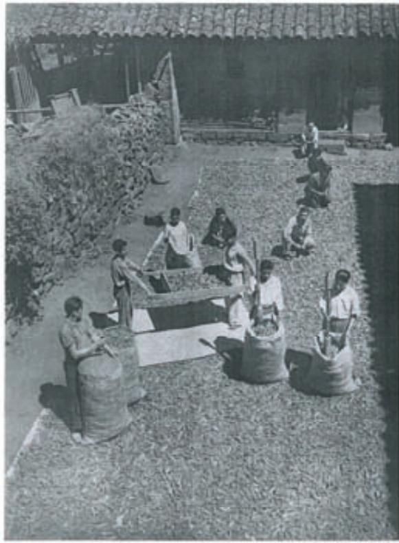
Workers Screen, Bag, and Tamp Sueded Bark at a Station in Baños
