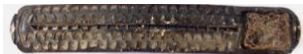
Fig. V-20. A no clogged non-pressure compensating emitter at 2/3 of lateral length from SDI system with root intrusion.
