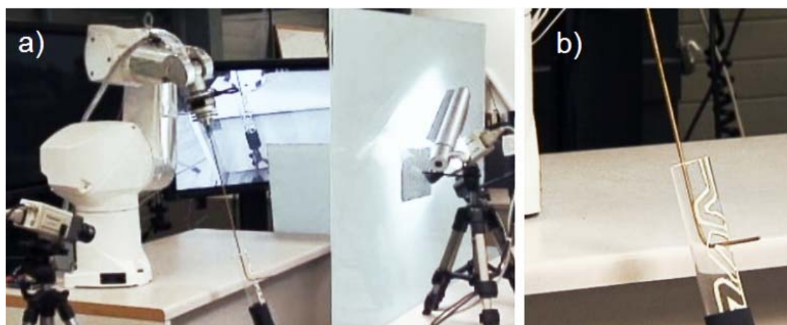
Figure 6.6. The workspace of the experimental setup simulated the remote environment which was composed by: a) A robot arm with a line-form object attached to its end-effector and two orthogonally located cameras; b) A cylinder with a carved curved route, which represented the operative site.
