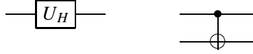
Figure 1: Quantum circuits representing the action of a Hadamard gate on a single qubit and a controlled-not gate on two qubits. The controlling qubit is denoted by a black dot, and the controlled qubit is denoted by the symbol \oplus .
