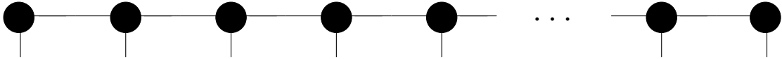
Figure 5.3: Diagrammatic representation of a matrix product state in terms of a tensor network.
