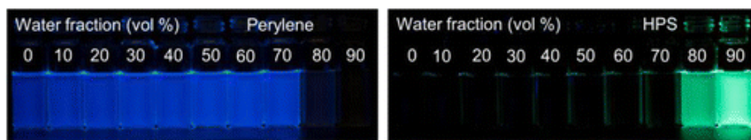
Figure 2.1 Fluorescence photographs of solutions or suspensions of (left) perylene (20 \mu\text{M} ) and (right) HPS (20 \mu\text{M} ) in THF/water mixtures with different fractions of water ( f_w ), with perylene and HPS showing typical ACQ and AIE effects, respectively. Taken from reference 5.
