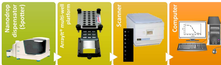
Figure 4.8. All material needed for the different steps involved in fluorescent microarray development: print, assemble, measure, analyze and data treatment.
