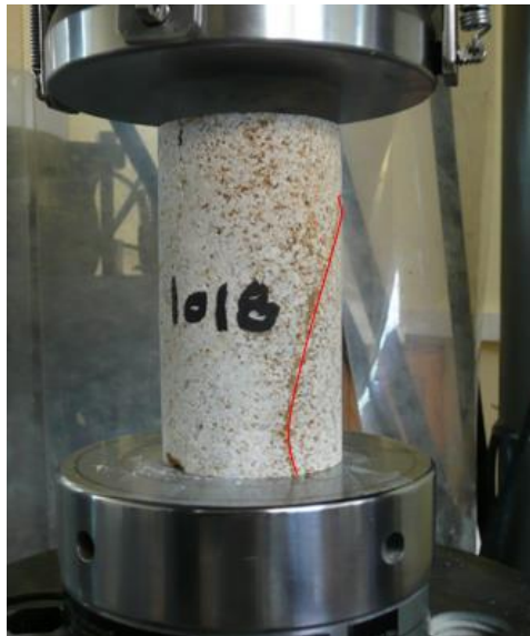
Figure 3-1 Discontinuity in sample 1018
