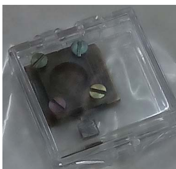
Figure 3. 6 \text{UO}_2 sample into the XPS sample holder before being introduced into the SPECS platform
