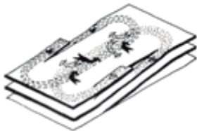
Fig. 5.44. Parallel Straight Ramp System. Measured in an automobile-parking deck on a ramp 65 feet long with a banked 180° turn at the top of the ramp and a partially banked 90° turn at the bottom, the up movements ranged from 5 to 9 sec, the down movements from 4 to 7 sec. The greater time required for the up travel may be accounted for by the approach to the blind turn at the top of the ramp; for down travel, this turn has been negotiated before the car reaches the ramp. Such physical differences in ramps will greatly affect operating time on the ramp.
