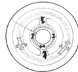
Fig. 5.55. "The 'Side' Garage. The general form of the side is characterized by an access-ramp in the form of a rising helix with parking space on both sides, turning about a central axis, and concentrically surrounding a helical exit-ramp which in turn surrounds the central opening. There is at least one point of tangency per floor (on both sides of the helix) between the access and exit ramps, thereby making it possible for departing automobiles to turn on to the exit ramp at every complete turn of the access helix. The exit ramp can be either continuously contiguous to the access ramp, or it can have in the opposite sense."
