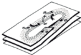
Fig. 5.43. Two-way Straight Ramp System.
