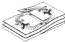
Fig. 5.47. Two-Way Staggered Floor Ramp System.
