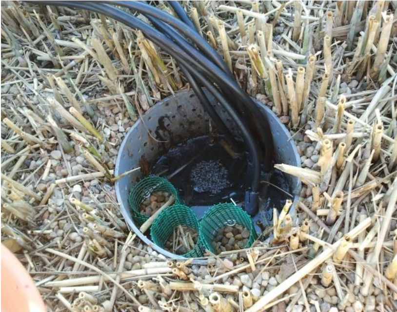
Figure 4.2.1 Microbial fuel cells implemented within the wetland at the beginning of the experiment.
