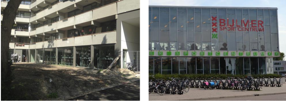
Figure 4.69: Example of the location of the bicycle parking's to encourage spontaneous surveillance
