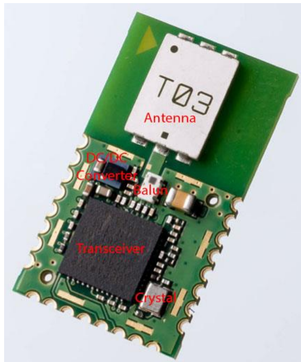
Figure 1.2 An indoor-location tag: DWM1000 module is based on a 90 nm CMOS IC TRx, integrated with a dielectric-chip antenna, DC/DC converter and xOSC on-board. Edited figure from [10].
