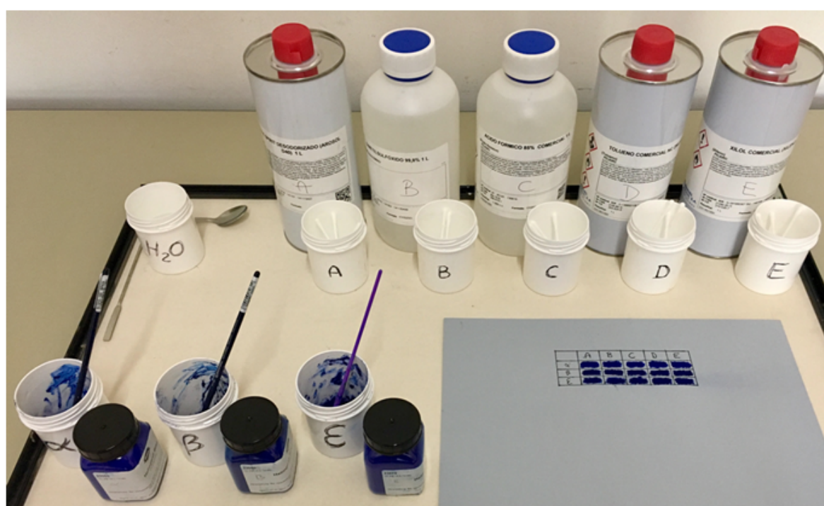
Figure 6.8: Experimental samples preparation using different polymorphic forms of copper phthalocyanine blue under solvents and cleaning agents
