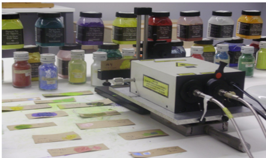
Figure 4.7: Measurement of experimental Raman spectra from handmade samples used for assessing the performance of the implemented identification methodology
