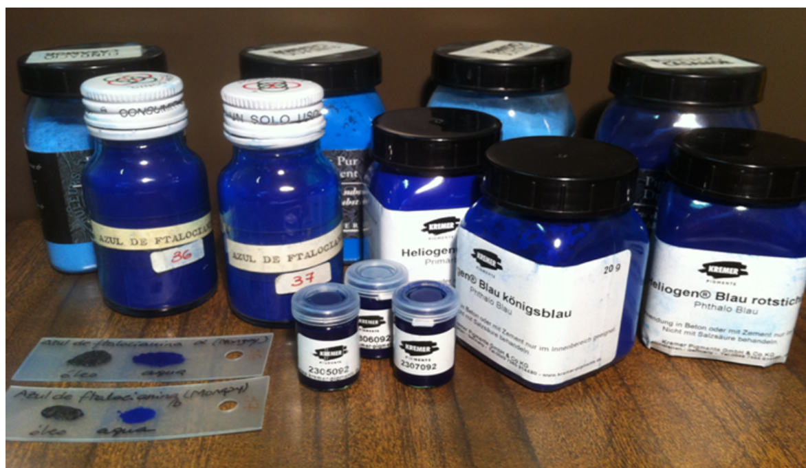
Figure 6.2: Pigment powders and hand-made samples from different crystalline structures of copper phthalocyanine blue
