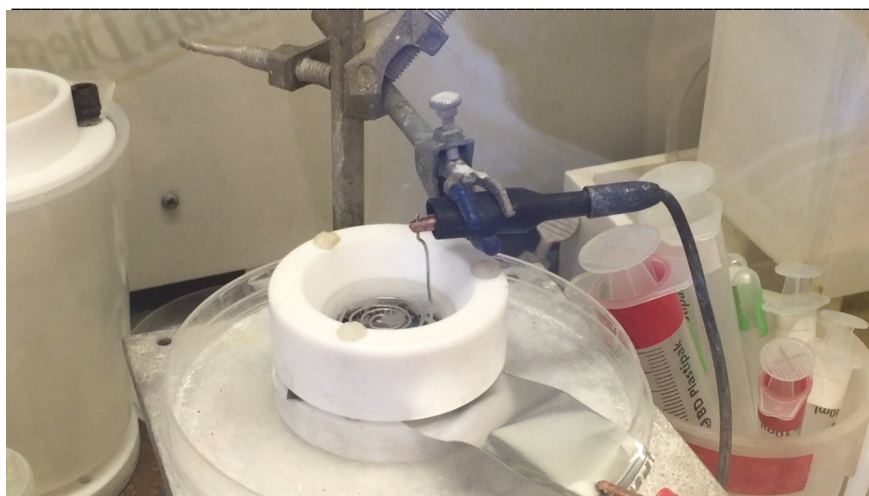
Figure 6.3. Image of an electrochemical etching of silicon in the current regime where porous silicon is formed. Hydrogen gas bubbles can be observed in the solution. This image was taken in Sailor's lab in University of California San Diego.
