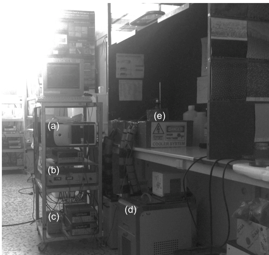
Figure 3.1. Experimental equipment required for the fabrication of NAA films. a) Personal Computer b) Power supply for anodization c) Power supply for the stirrer d) Cooling system e) Anodization cell
