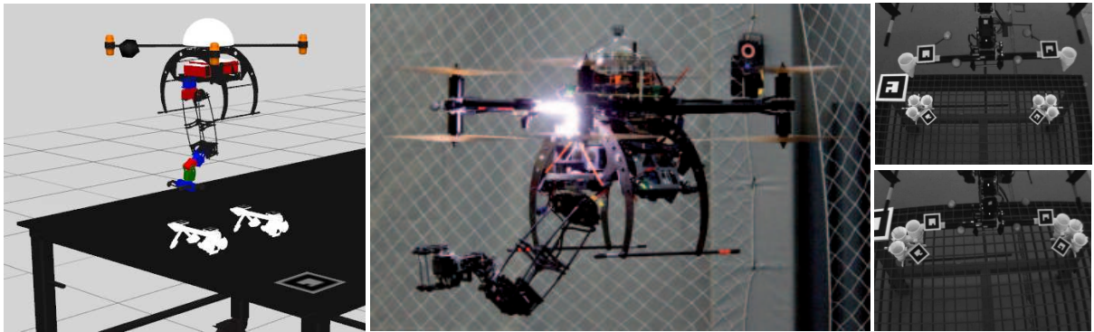
Figure 4.3: Bonebraker UAM employed during the simulations (left) and real experiments (middle), and images from the on-board camera during the approaching phase (top-right) and at the plugging instant (bottom-right).
