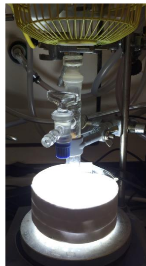
Figure 3.5 Reaction set up under irradiation of white LEDs
