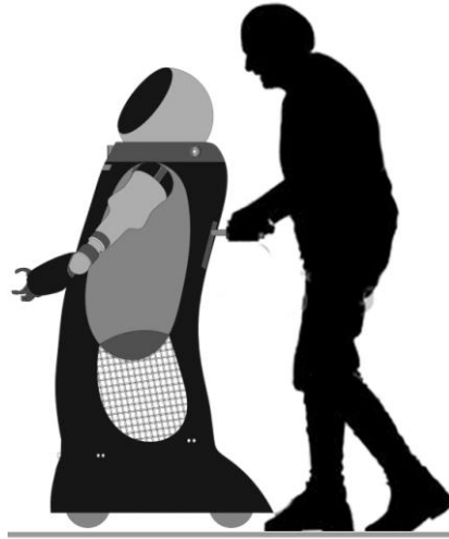
Figure 47 Mobile servant robot size and avoidance of the “poor visibility” hazard
