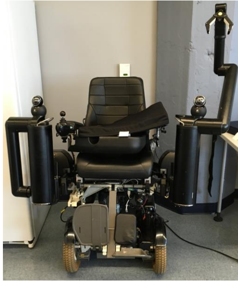
Figure 61 Wheelchair with Robotic Arm from the Human Engineering Research Laboratory (HERL) Center at the University of Pittsburgh 1174
