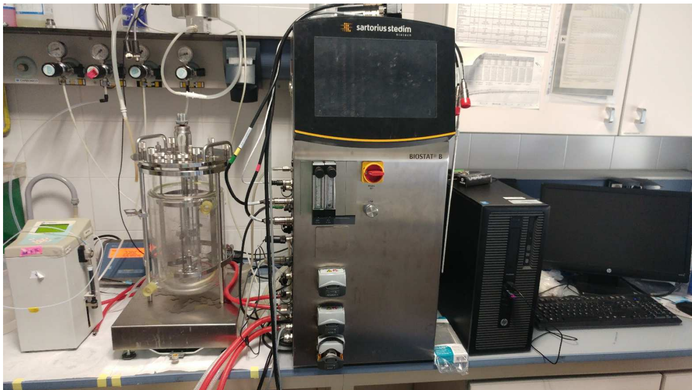
Figure 3.5 Bench-top bioreactor (Biostat B) full equipment to produce RPP by Pichia pastoris . From left to right, a microburette, the vessel of the bioreactor, the DCU and the PC for supervision, control and data acquisition.
