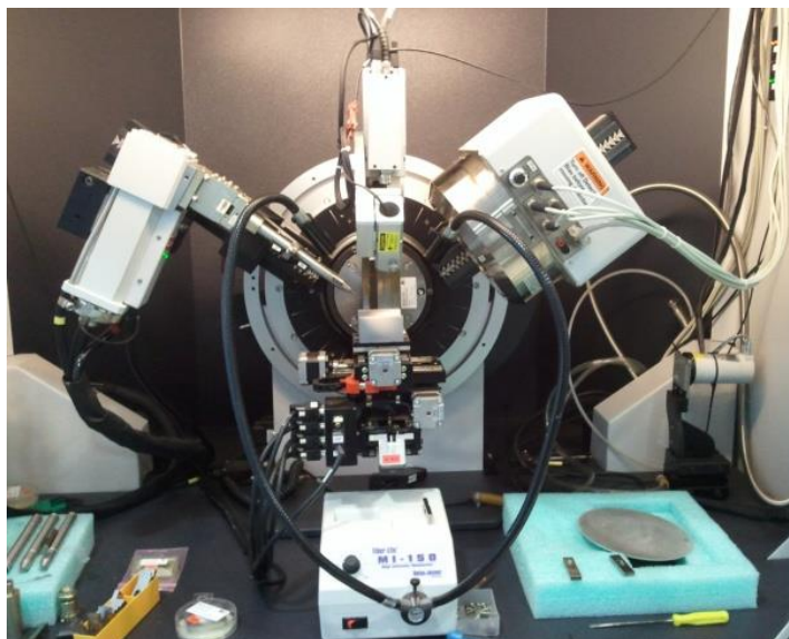
Figure 2.14. Bruker-AXS D8-Discover diffractometer used in this thesis.
