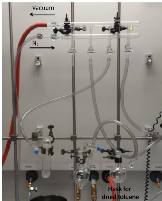
Figure 2.8. Experimental setup of the Schlenk line for drying and removing oxygen from the reaction flasks.
