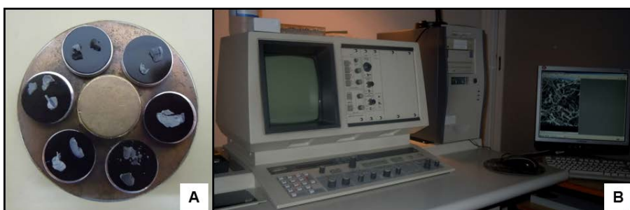
Figure 2. Computer scanning electron microscopy. (A) Samples after coating with gold, (B) Scanning Electron Microscope Hitachi S-70, used for the evaluation of the different samples.
