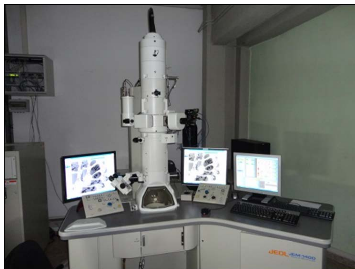
Figure 3. Transmission Electron Microscope JEOL JEM,-1400, used for the evaluation of the different samples.
