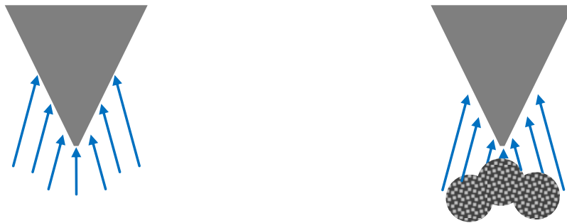
Figure 4.10. Averaging effect of the CPD signal by measuring nanoscale grains and interspaces.
