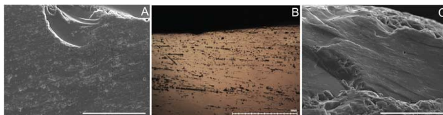
Fig. 7. Furrow striations after sawing wood. A), quartz, orig. mag.: 1000×, scale bar: 50 µm; B) rock crystal, orig. mag.: 500×, scale bar: 100 µm; C) quartzite, orig. mag.: 1000×, scale bar: 50 µm.
