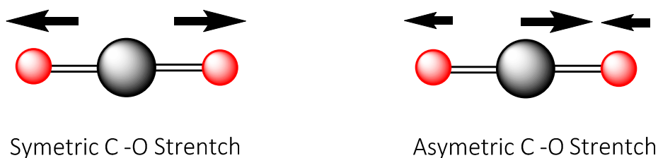
Figure 2.13. Raman active (left) and IR active (right) vibrations of carbon dioxide.
