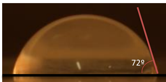
Figure 8.4. Example of contact angle measurement from water drop photograph (polyurethane sample coated with electrospun crosslinked fibers).
