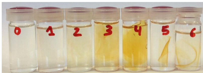
Figure 7.8: Physical state of the gelatin films (FA0-FA6) after the immersion in water for 5 days
