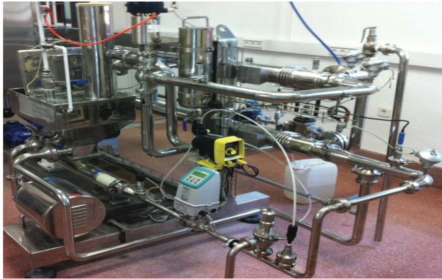
Figure 7.3 Photograph of the pilot plant containing the in-line pH control system
