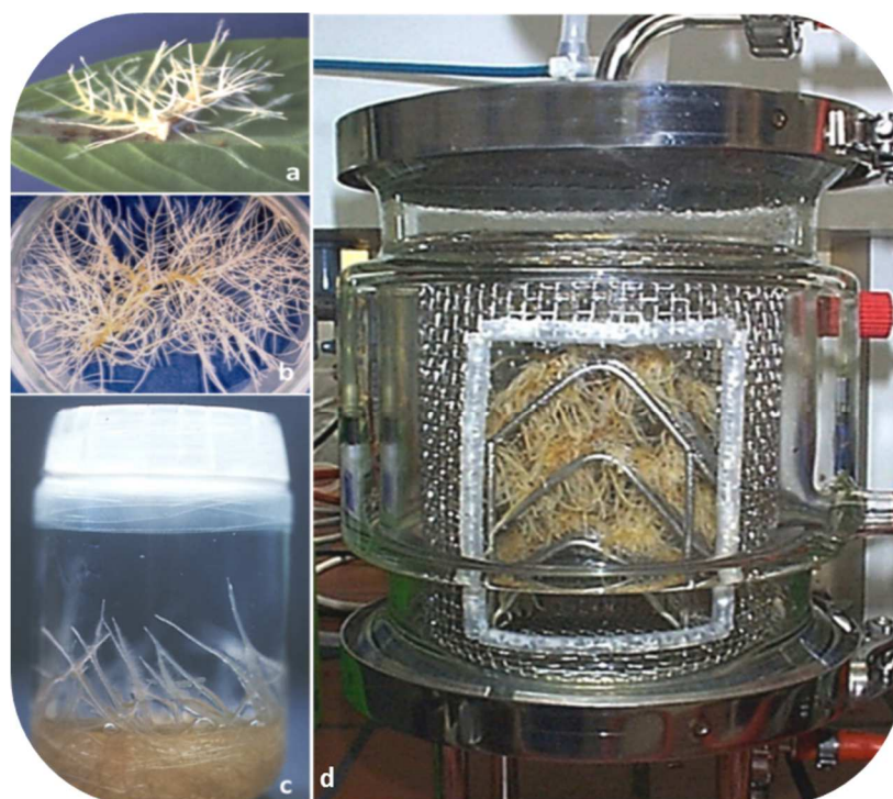
Fig. 3. Sequential steps to develop a plant biofactory based on hairy root culture platforms. a) root induction; b) root line isolation; c) root culture; d) bioreactor culture.
