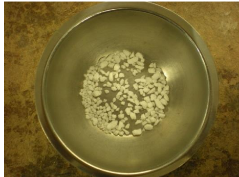
f. Particles retained in Sieve # 10 - 2.0mm
