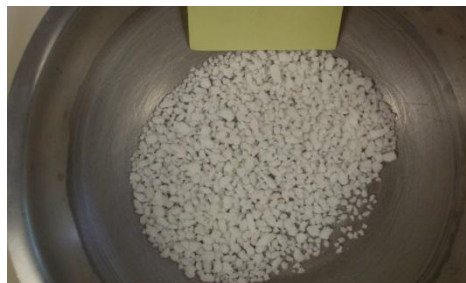
f. Particles retained in Sieve # 10 - 2.0mm
