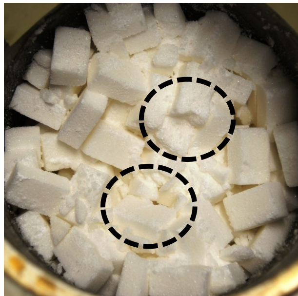
Figure 4-20 Local or Comminution crushing.
