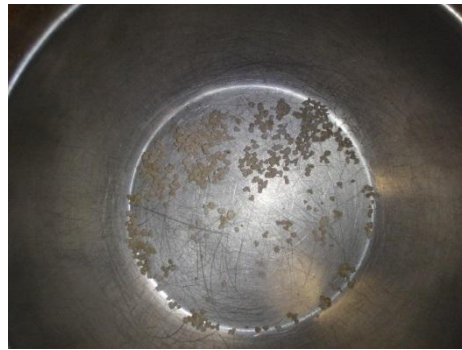
g. Particles retained in Sieve # 16 - 1.18mm
