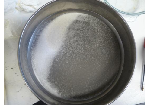
j. Particles retained in Sieve # 200 - 0.075mm
