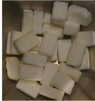
a. Intact Particles: Retained in Sieve 1/2"- 12.1mm
