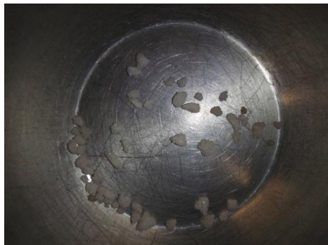
f. Particles retained in Sieve # 10 - 2.0mm
