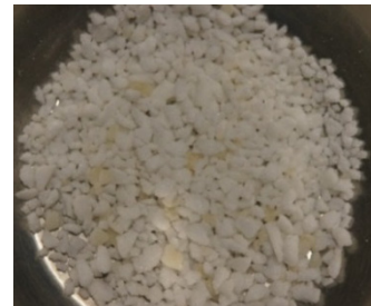
f. Splitting Crushing: Retained in Sieve # 10 - 2.0mm
