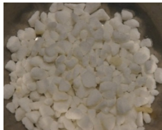
e. Splitting Crushing: Retained in Sieve # 4 - 4.75mm
