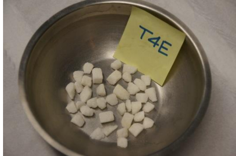
d. Particles retained in Sieve 3/8"- 9.5mm
