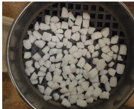
d. Particles retained in Sieve 3/8"- 9.5mm
