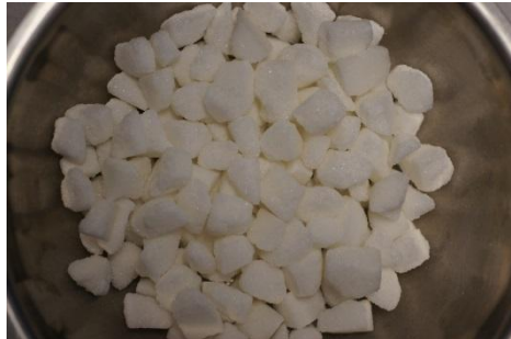
d. Particles retained in Sieve 3/8" - 9.5mm
