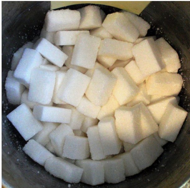
Figure 4-9 Disordered arrangement sample ( e_0 = 0.78 ) inside the oedometer cell (diameter 152mm).
