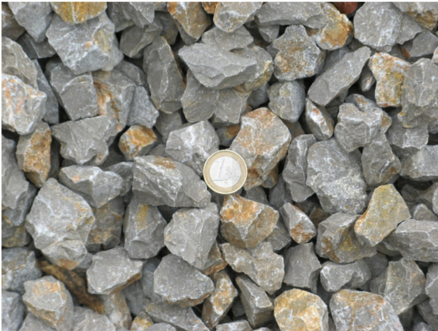
Figure 5-9 Hard limestone gravels from a quarry in Vallirana (Barcelona, Spain). Material tested by Ortega (2008).
