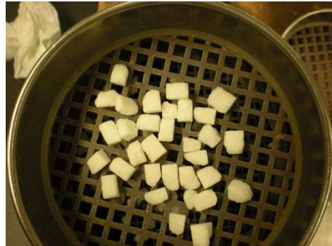
d. Particles retained in Sieve 3/8" - 9.5mm
