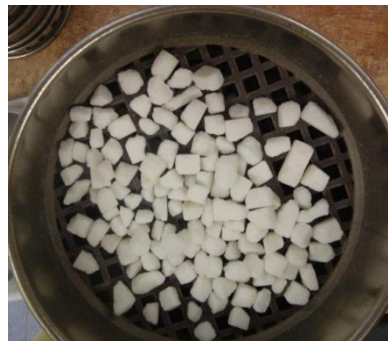
d. Particles retained in Sieve 3/8"- 9.5mm
