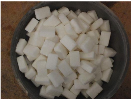
a. Intact particles: Retained in Sieve 1/2"-12.1mm
