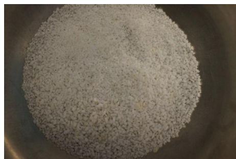
g. Particles retained in Sieve # 16 - 1.18mm
