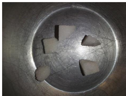
d. Particles retained in Sieve 3/8"-9.5mm
