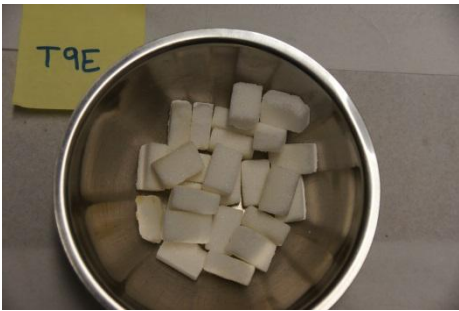
a. Intact particles: Retained in Sieve 1/2" - 12.1mm
