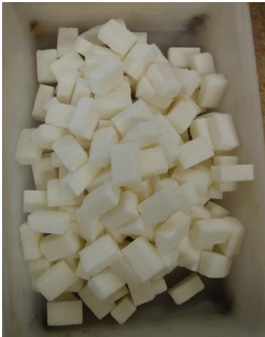
a. Intact particles: Retained in Sieve 1/2"- 12.1mm
