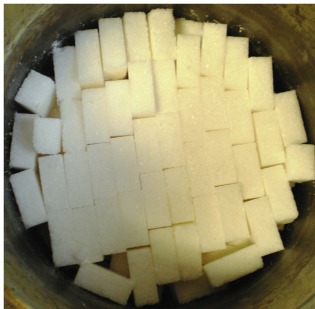
Figure 4-8 Ordered arrangement sample ( e_0=0.18 ) inside the oedometer cell (diameter 152mm).
