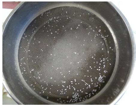
g. Particles retained in Sieve # 16 - 1.18mm
