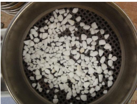
e. Particles retained in Sieve # 4 - 4.75mm
