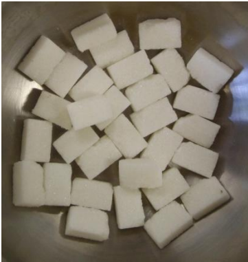
a. Intact particles: Retained in Sieve 1/2"- 12.1mm
