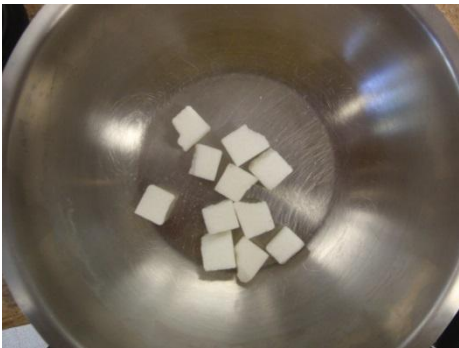
c. Splitting crushing: Retained in Sieve 1/2"- 12.1mm
