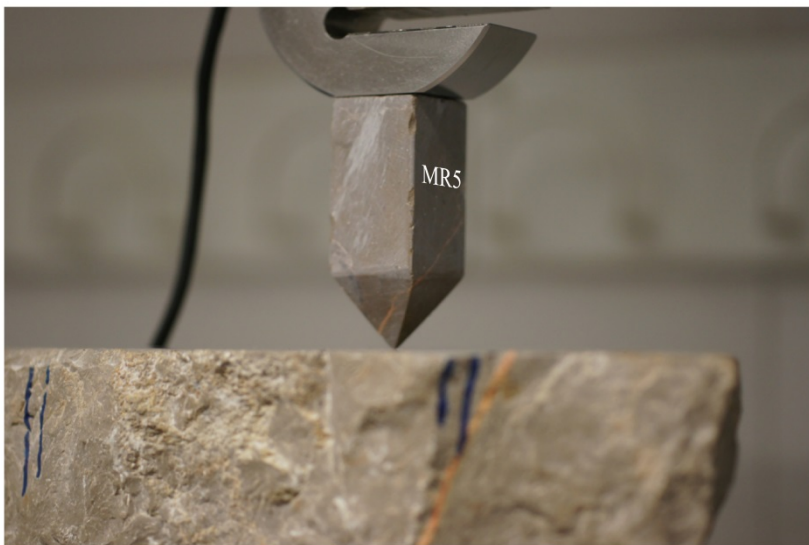
Figure 5-23 a) Limestone samples for contact stiffness tests: MR1, MR2, and MR3 ( 90^\circ apex angle); MR4, MR5 and MR6 ( 70^\circ apex angle). Height of samples: 6 cm; Cross section: 2.5 cm x 2.5 cm; b) detail of testing arrangement.
