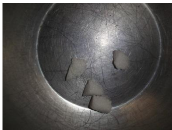
e. Particles retained in Sieve # 4 - 4.75mm
