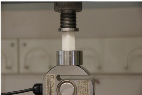
Figure A4 - 9 Simple compression tests on the CS7-sugar cube sample.
