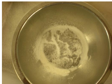
i. Particles retained in Sieve # 100 - 0.15mm
