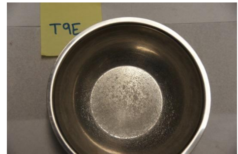
j. Particles retained in Sieve # 200 - 0.075mm
