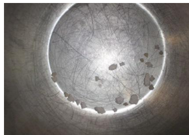
f. Particles retained in Sieve # 10 - 2.0mm
