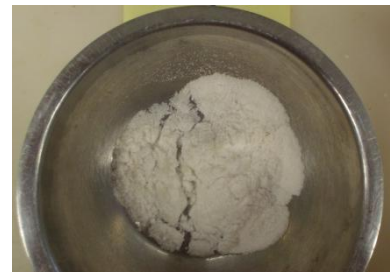
j. Particles retained in Sieve # 200 - 0.075mm
