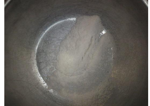
j. Particles retained in Sieve # 200 - 0.075mm
