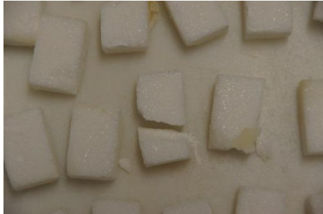
f. Details of broken particles of sample T8E: Splitting (center) and Comminution (right)
