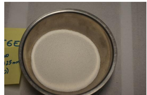
h. Particles retained in Sieve # 40 - 0.425mm (Sugar Crystals)
