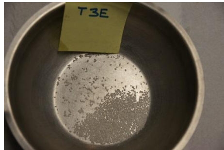
g. Particles retained in Sieve # 16 - 1.18mm
