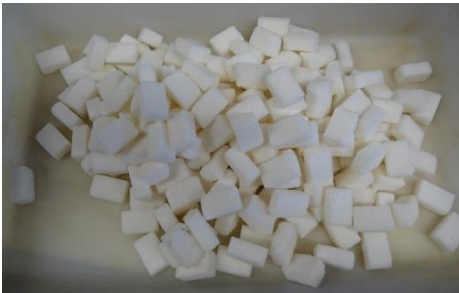
a. Intact particles: Retained in Sieve 1/2"- 12.1mm
