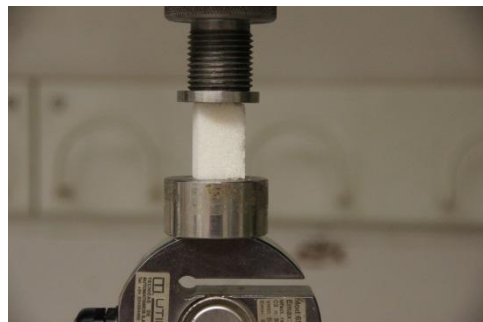
Figure A4 - 6 Simple compression tests on the CS4-sugar cube sample.
