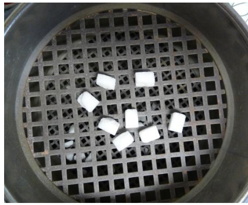
d. Particles retained in Sieve 3/8"- 9.5mm
