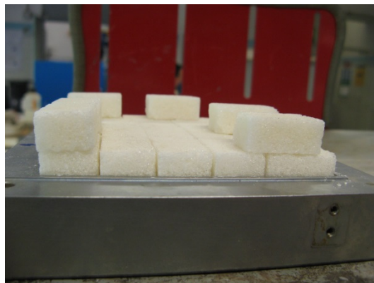
Figure 4-6 M2A slider arrangements (individual sugar cubes). Tilting table test: sliders over a plate block.
