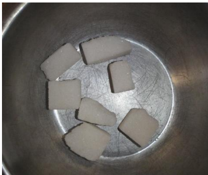
c. Splitting crushing: Retained in Sieve 1/2"-12.1mm
