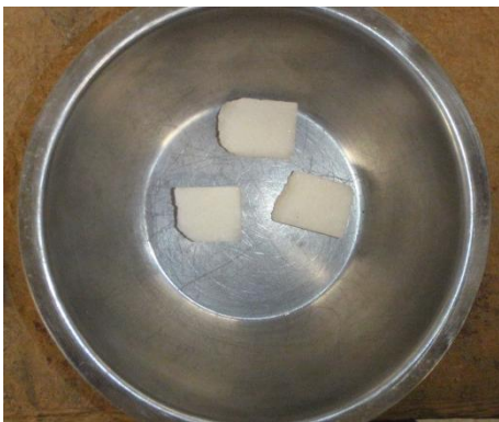
c. Splitting crushing: Retained in Sieve 1/2"- 12.1mm
