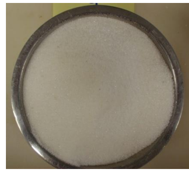
h. Particles retained in Sieve # 40 - 0.425mm (Sugar Crystals)
