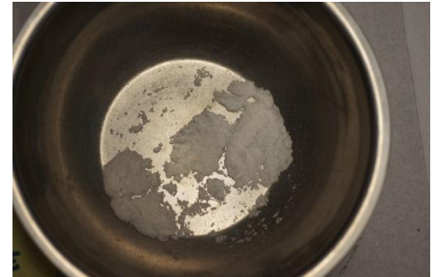
j. Particles retained in Sieve # 200 - 0.075mm
