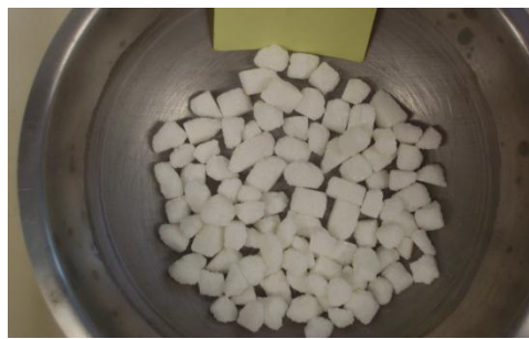
d. Particles retained in Sieve 3/8" - 9.5mm
