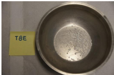
f. Particles retained in Sieve # 10 - 2.0mm
