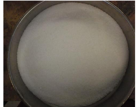
h. Particles retained in Sieve # 40 - 0.425mm (Sugar Crystals)
