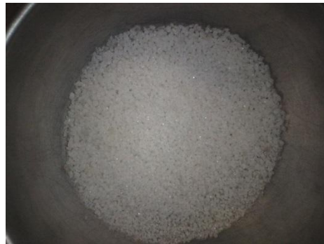
g. Particles retained in Sieve # 16 - 1.18mm
