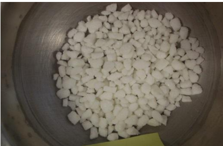
e. Particles retained in Sieve # 4 - 4.75mm
