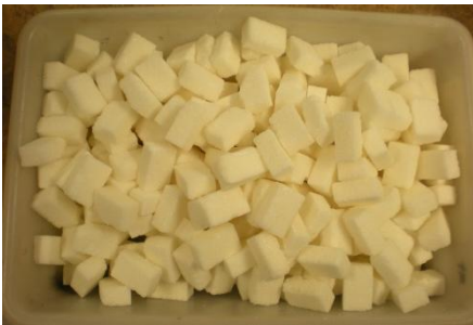
a. Intact particles: Retained in Sieve 1/2" - 12.1mm
