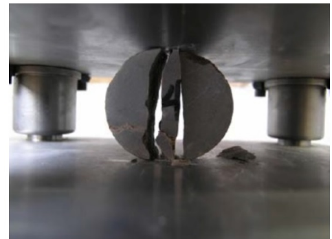
b. Brazilian test on limestone particle (From Ortega (2008)).
