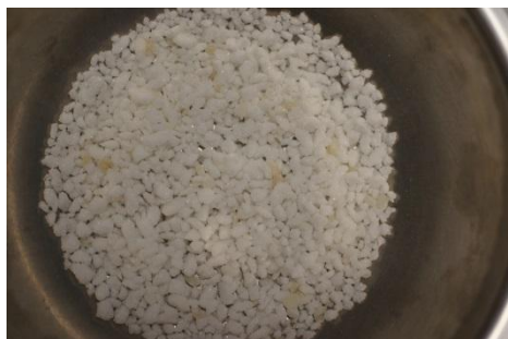
f. Particles retained in Sieve # 10 - 2.0mm
