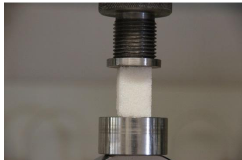
Figure A4 - 8 Simple compression tests on the CS6-sugar cube sample.
