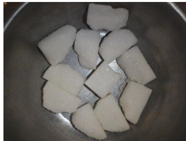
b. Particles with local crushing: Retained in Sieve 1/2"- 12.1mm
