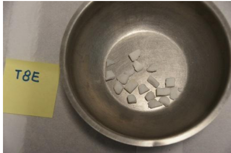
d. Particles retained in Sieve 3/8" - 9.5mm
