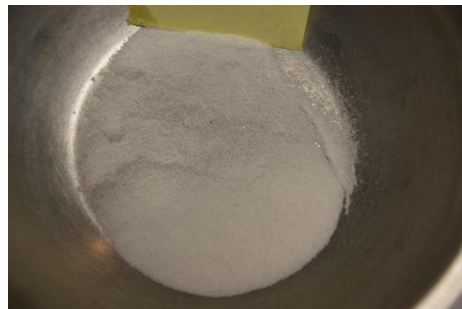
i. Particles retained in Sieve # 100 - 0.15mm
