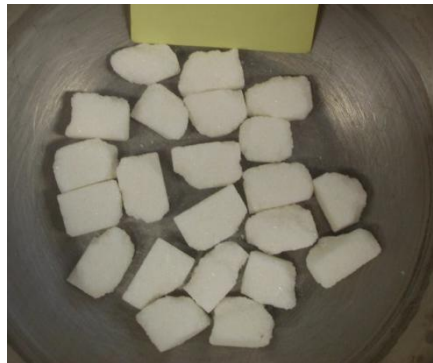
b. Particles with local crushing: Retained in Sieve 1/2" - 12.1mm
