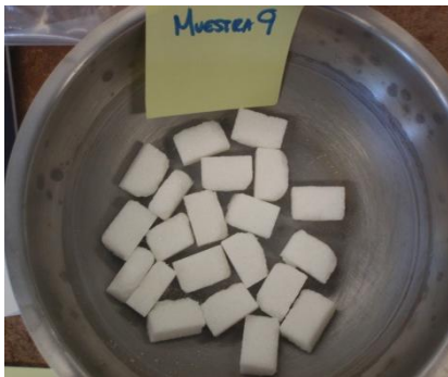
a. Intact particles: Retained in Sieve 1/2"- 12.1mm
