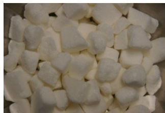
c. Splitting Crushing: Retained in Sieve 1/2"- 12.1mm
