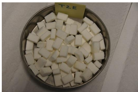
a. Intact particles: Retained in Sieve 1/2" - 12.1mm
