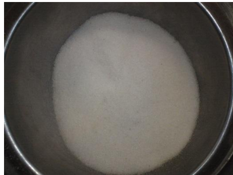
i. Particles retained in Sieve # 100 - 0.15mm
