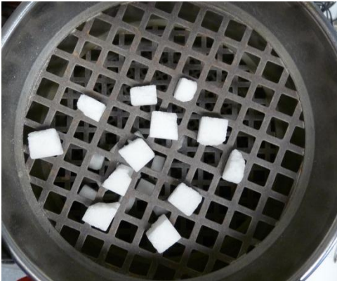
c. Splitting crushing: Retained in Sieve 1/2"- 12.1mm
