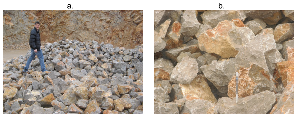
Figure A5 - 1 Limestone rockfill from the quarry FOJ in Vallirana (Barcelona, Spain): (a) Particle size: 0.1 – 0.5m; (b) Detail of rock fragments.
