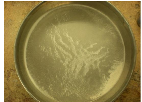
j. Particles retained in Sieve # 200 - 0.075mm
