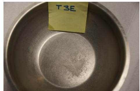
j. Particles retained in Sieve # 200 - 0.075mm
