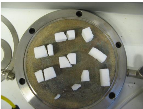
a. Details of broken particles of sample M1
