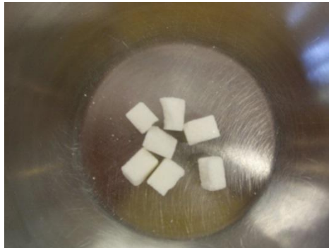
d. Particles retained in Sieve 3/8" - 9.5mm
