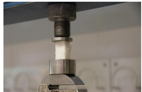
Figure A4 - 3 Simple compression tests on the CS1-sugar cube sample.
