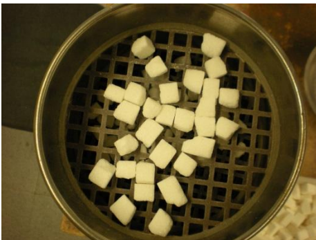
c. Splitting crushing: Retained in Sieve 1/2" - 12.1mm
