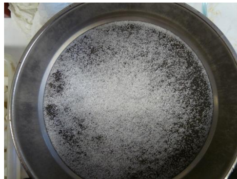
i. Particles retained in Sieve # 100 - 0.15mm
