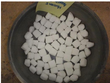
c. Splitting crushing: Retained in Sieve 1/2"- 12.1mm
