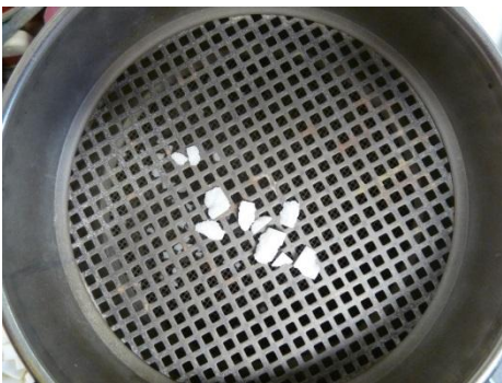
e. Particles retained in Sieve # 4 - 4.75mm
