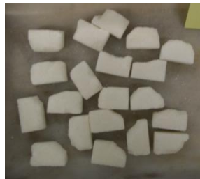
b. Particles with local crushing: Retained in Sieve 1/2"- 12.1mm
