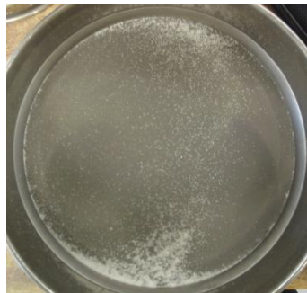
i. Particles retained in Sieve # 100 - 0.15mm
