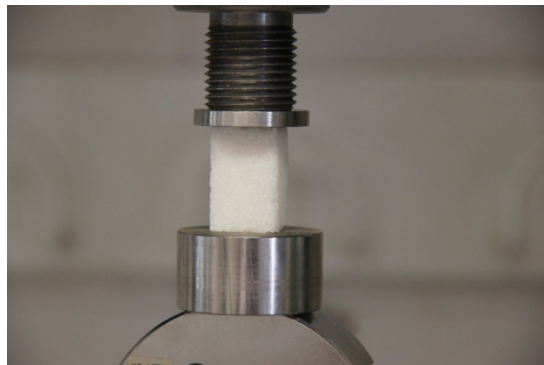
Figure 4-3 Simple compression tests on sugar cube samples.
