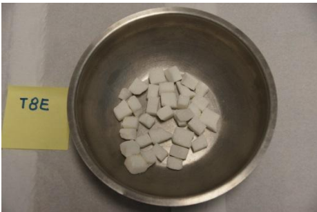
c. Splitting crushing: Retained in Sieve 1/2" - 12.1mm
