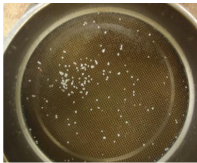
g. Particles retained in Sieve # 16 - 1.18mm
