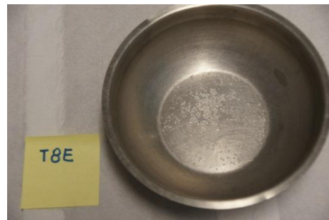
g. Particles retained in Sieve # 16 - 1.18mm
