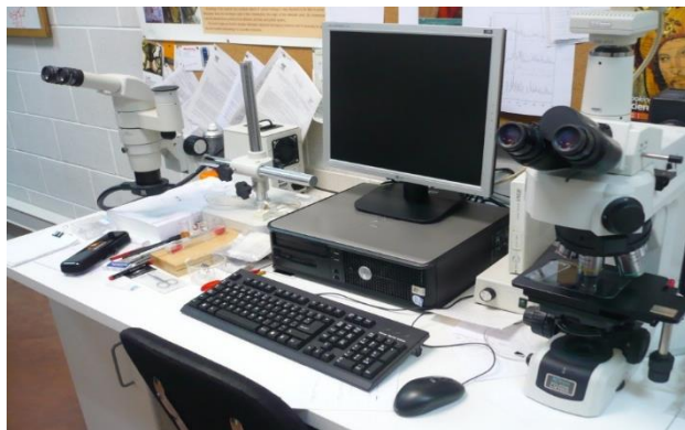
Figure 2.3 Stereomicroscope Nikon SMZ800 (left) and optical microscope Nikon Eclipse LV100 (right).
