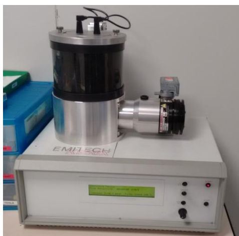
Figure 6.1 Turbo evaporator Emitech K950X from Centre de Recerca en Nanoenginyeria CRnE (UPC).
