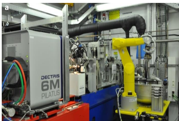
Figure 2.8 a) Beamline XALOC from ALBA-CELLS, b) Beam of 6 \times 50\ \mu\text{m} used for \mu SR-XRD.
