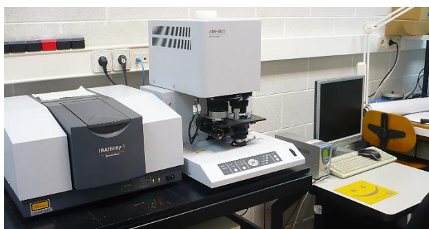
Figure 2.1 Microscope AIM-8800 with a MCT detector coupled to the Shimadzu IRAffinity -1 FTIR spectrometer.
