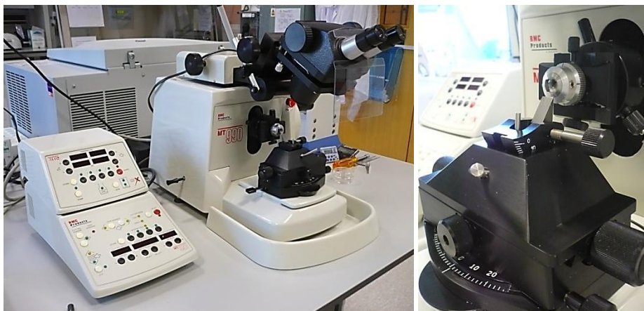
Figure 6.2 Motorized Rotary Microtome RMC MT-990 from Diamond Light Source (UK).
