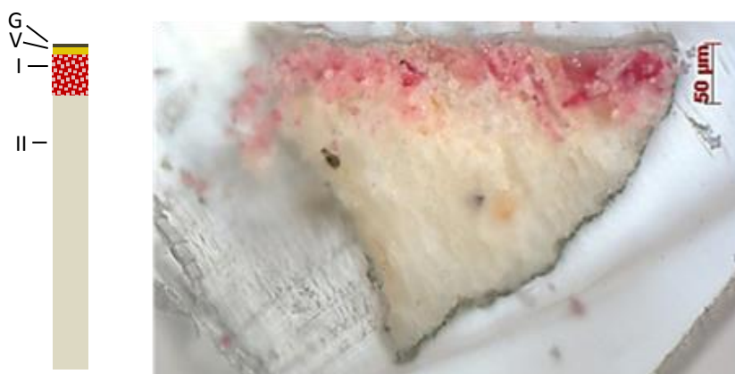
Figure 6.19 Scheme of the layers, G: gold coating, V: varnish, I: chromatic layer, II: preparation layer (right) and thin section of the sample by OM with polarized light (left).
