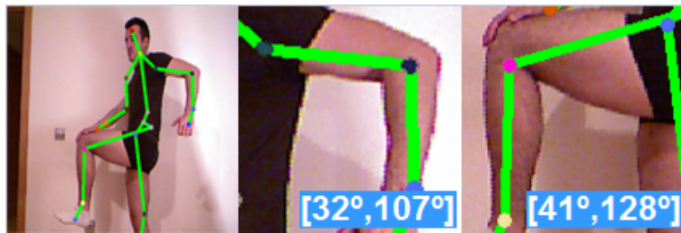
Figure 2.13: Skeletal model and example of selected articulations with computed dynamic range of movement (maximum opening and minimum closing values of a joint measured in degrees for a certain period of time).
