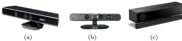
Figure 1.1: Example of the variability of low-cost and compact RGB-D devices. (a) Kinect first version launched in November 2010 by Microsoft Corp. RGB Resolution: VGA 640x480, Depth resolution: 320x240 (b) RGB-D camera launched in July 2011. RGB Resolution: SXGA 1280x1024, Depth resolution: 320x240. (c) Kinect second version launched in July 2014 by Microsoft Corp. RGB Resolution: HD 1080x1920, Depth resolution: 620x480.
