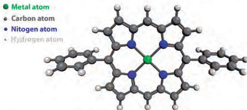
Figure 3.5: Representation of the Co-metalloporphyrin (Co-DPP) used in this study, atoms are labeled on the figure.
