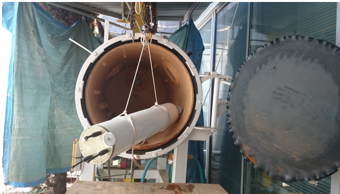
Figure 5.14: Water tight cylinder enclosing cRIO based acoustic modem electronics
