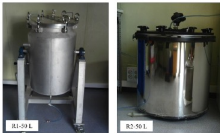
Figure 3.5. Picture of pilot reactors of 50-L of working volume.
