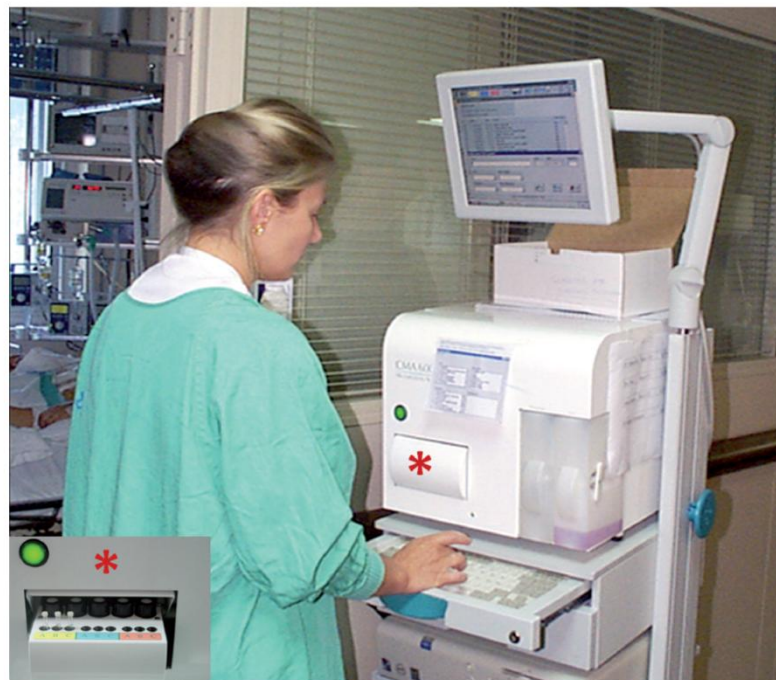
Figure 100-2. Analysis of the microvials performed by the nurse using the portable analyzer placed at the bedside. The different metabolites are determined using enzymatic techniques.
