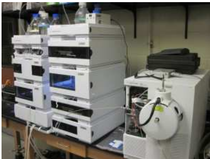
Figure 3.5: Agilent gas Chromatograph flame ionizator detector coupled to an Agilent gas chromatograph with a single quadrupole mass spectrometer from the Dr. Timothy Shanahan laboratory at the University of Texas at Austin. This instrument is used for the lipid identification and quantification.
