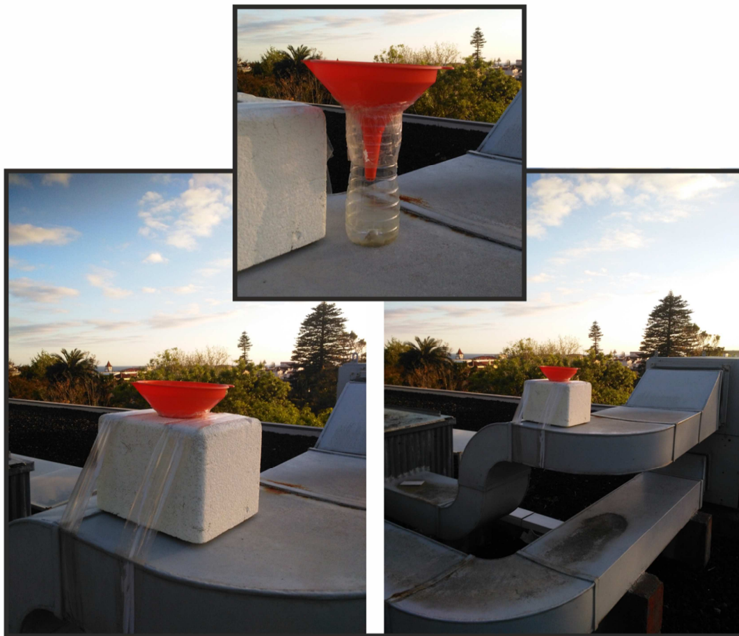
Figure 3.7: Rain water collector located at the University dos Açores. The upper figure shows the internal structure of the water collector. The lower pictures showed the collector cover made of porexpan® to avoid evaporation and the location without any shadow effect of the collector.
