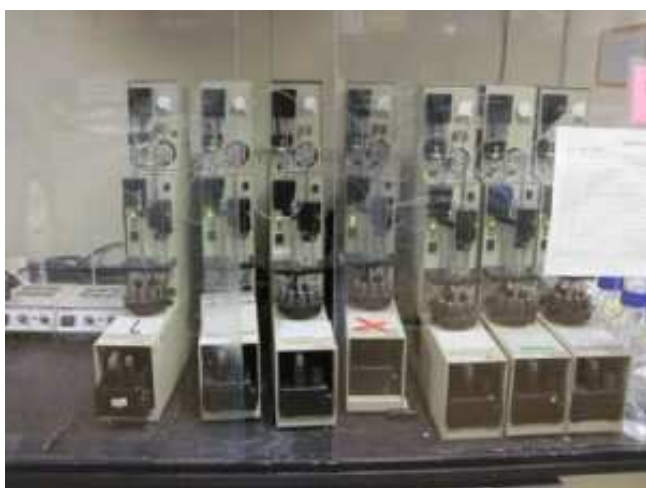
Figure 3.4: Specialized vented cabinet used for a total of 7 Zymark Rapid Traces at the Dr Timothy Shanahan laboratory at the University of Texas at Austin. This rapid trace can separate chromatographically lipid fractions from the extracted lipids.
