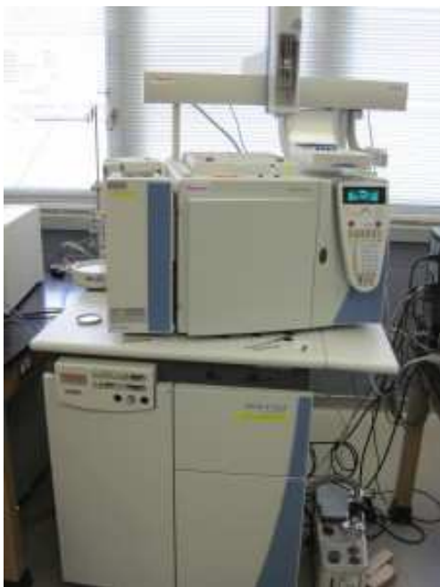
Figure 3.6: Delta V stable isotope mass spectrometer from the Dr Shanahan laboratory at the University of Texas at Austin. This IRMS is equipped with a combustion furnaces for hydrogen, carbon and nitrogen isotope analyses from molecular organics.
