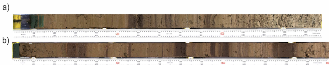
Figure 3.3: The high resolution photographs of studied Azul cores. (a) core AZ11_02; (b) core AZ11_14). Images were obtained from CCD color line scan camera with RGB channels at 630, 535 and 450 nm mounted on an Avaatech. The iris aperture was 5.6 for picture (a) and 5.6+ for picture (b). The top of the sequence is on the left.
