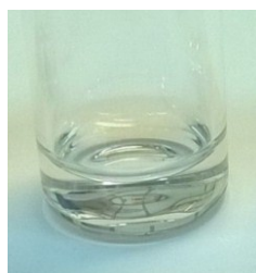
Figure 4.1 – Vial with the reaction components dissolved in MTBE at the same concentration employed for carrying out the reaction: aldehyde 20 (1.5 M), catalyst IV (0.1 M), 2,6-lutidine (0.5 M) and diethyl bromomalonate 21 (0.5 M) in MTBE.
