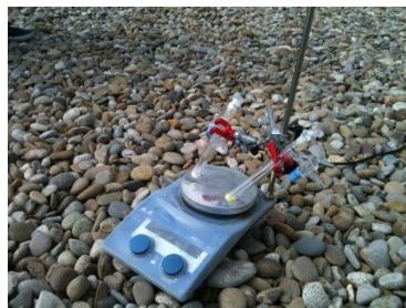
Figure 4.14 The simple set-up for the sunlight-driven reaction.
