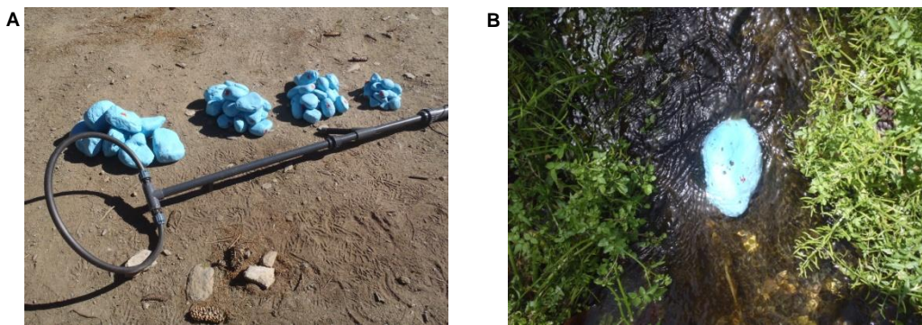
Figure 21. (A) Example of the tracers with a radio system (RFID) and the antenna; (B) Example of a tracer with a RFID in the River Siurana downstream from Siurana reservoir (SIU DS ).
