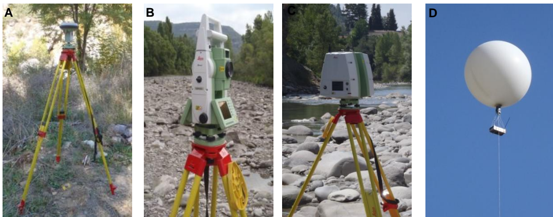
Figure 17. (A) Local Base or Reference GPS Station used to correct rtk-GPS-based observations (Leica® GNSS/GPS); (B) Leica® TCRP1201 Robotic Total Station; (C) Terrestrial Laser Scanning Leica® ScanStationC10; (D) Digital camera attached to a helium balloon to acquire close range aerial photographs.
