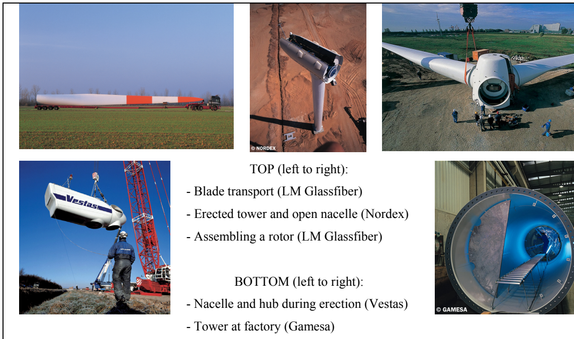
Figure 8: Hub, nacelle and blades
