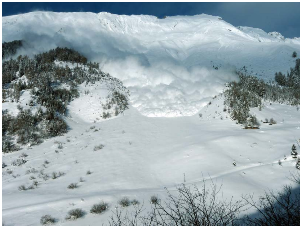
FIGURE 4.1: Image of a typical powder-snow avalanche at VdlS released in the experiment on 3rd February 2015. The avalanche was triggered by an explosion from the PR area and most of the mass flowed over gully 1 and the rest of the mass flowed through Deylon gully (see Figure 2.1). Photo courtesy of SLF.
