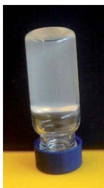
Figure 15. Picture of a vial turned upside down to check if a gel is formed.
