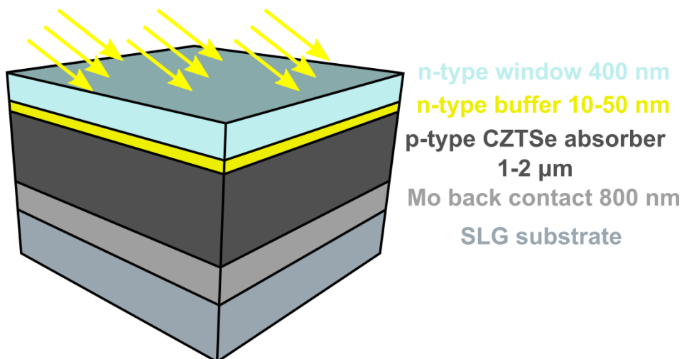
Figure 3.1. Schematic device structure of typical kesterite solar cell
