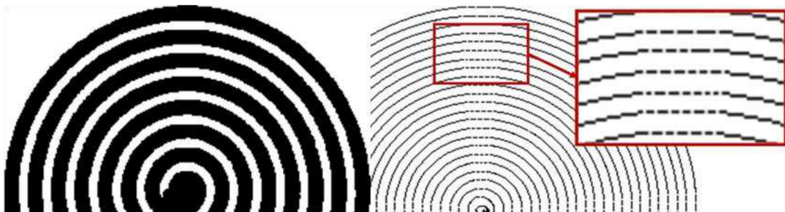
Fig. 4: Layout of a semi-spiral drawn for the inkjet printing process. On the left, the 11-pxl spiral and, on the right, the 1-pxl spiral. The number of pixels (drops) is reduced in those zones of ink accumulation.
