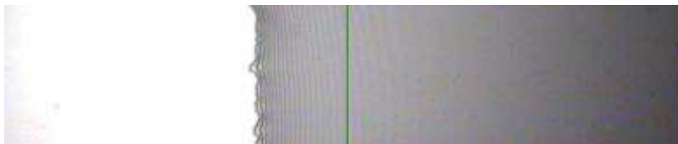
Fig. 10: Printed CZTS solution with a 1% wt. of leveling additive onto a Mo-covered glass substrate showing a full wetting.
