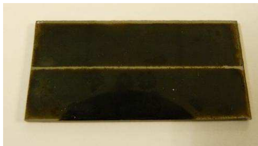
Fig. 12: Dried CZTS printing of two 2.5x5 cm dried at 280°C. This sample was printed with solution B.
