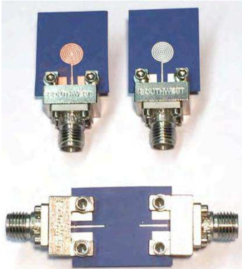
Fig. 24: Example of connectorized 6 turns spiral inductors fabricated using LTCC technology combined with inkjet printing and electroless growth (top left) and standard LTCC technology (top right). Connectorized open and short test structures used for de-embedding are also shown (bottom).
