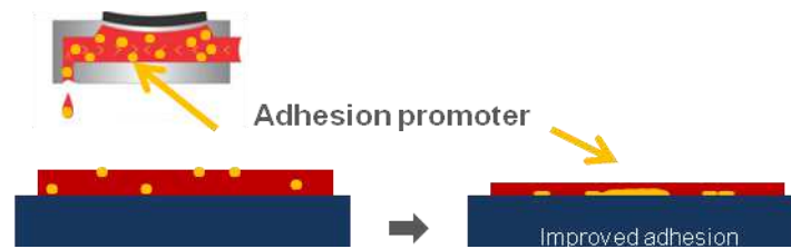
Fig. 33: The addition of some adhesion promoters such as glass frit inside the ink can strengthen the interaction between the ink and the substrate
