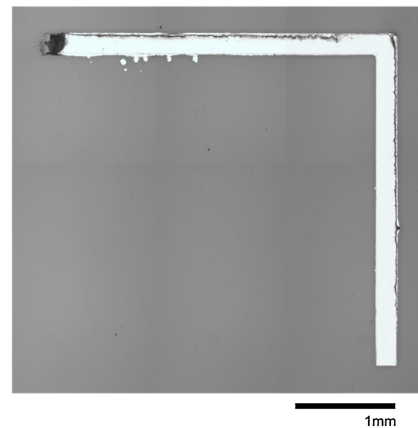
Fig. 5. a) Conductive lines generated by printing Ag ink through LIFT at different shifts between consecutive droplets (measured from center to center) inside fluidic guides with a constant width of 200 \mu\text{m} . b) Pattern consisting in two long and connected straight lines forming an angle of 90^\circ generated through LIFT of Ag ink inside previously ablated fluidic guides of 200 \mu\text{m} width.
