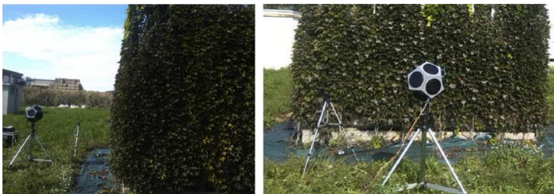
Figure 19. In situ acoustic measurements according to UNE-EN ISO 140-5
