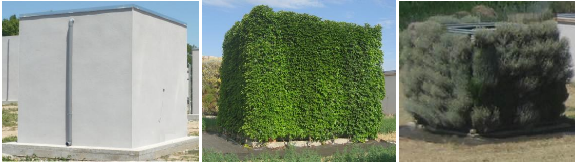
Figure 17. Studied cubicles in the experimental set-up in Puigverd de Lleida. From left to right: Reference, Double-skin green facade, and Green wall
