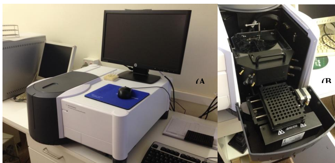
Figure 4.8. (A) Cary Eclipse Fluorescence Spectrophotometer (Agilent Technologies) (B) with a plate reading accessory.
