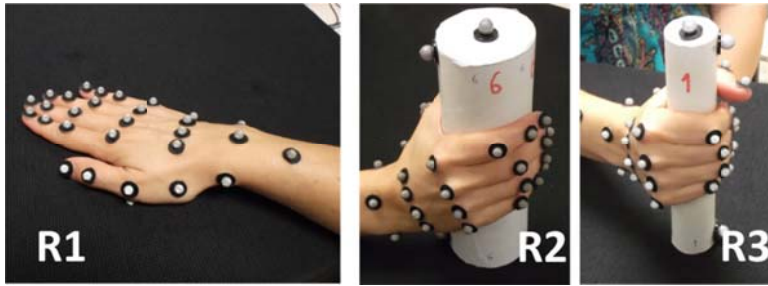
Figure 3.1. Reference postures: R1) hand lying on a flat surface (used as zero rotation angles), and R2) and R3) hand grasping cylinders with different diameters.
