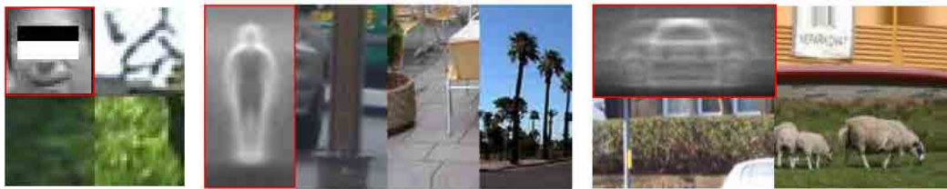
Figure 4.1: Figure taken from [Ram07]. Examples of false positives for a face detector (left), a pedestrian detector (middle), and a car detector (right) using scanning-window template classifiers.
