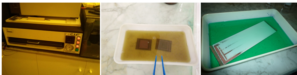
Figure C.3: Different images of the photo-etching technique: UV-exposure system (left), development of the array substrates (middle), and etching process (right), carried out at UPC facilities.
