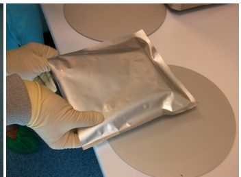
Figure C.9: Some parts of the LTCC process: hermetically sealed of the stacked layers (left and right photographs), and work space at the facilities of the UPV.
