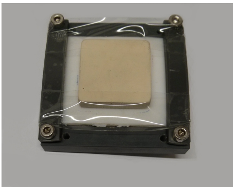
Figure 2.22: TMM6 sample of 7 mm thickness and its measured permittivity.
